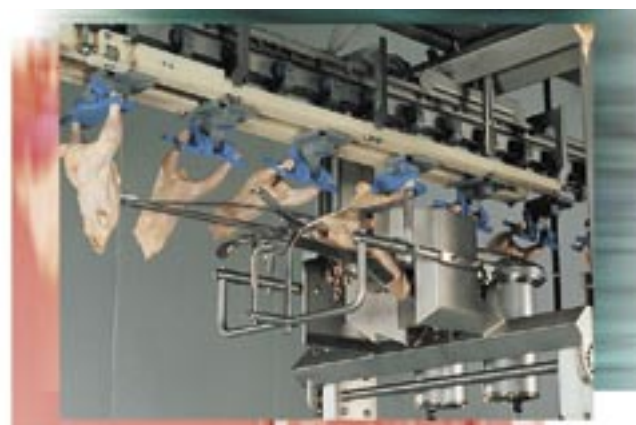
This 83 per minute poultry cutup machine was designed by a team of American and Dutch Mechanical Engineers. Used worldwide, these machines are manufactured by Stork PMT in Holland & Stork Gamco Inc. of Gainesville, Ga
