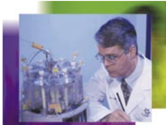
Biomedical engineer tests new heart valve surgical product using a machine to simulate the heart beating at 25 times normal rate. CryoLife, Inc., Kennesaw, Ga.
