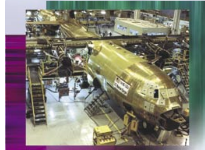
Aeronautical Engineers design aircraft and oversee the fabrication and assembly. 400 engineers and 1,600 other Lockheed Martin employees in Marietta, Ga. build twelve C130 military cargo planes per year.
