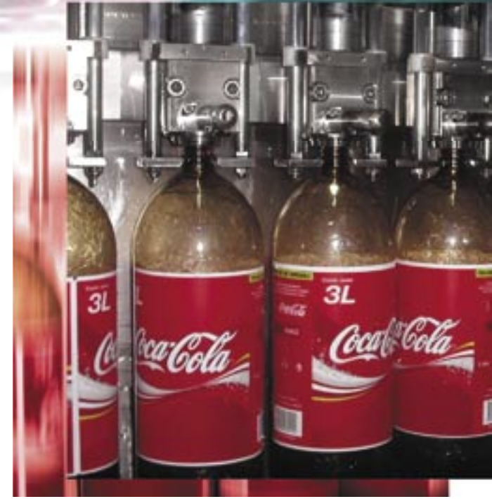
Mechanical and Electrical engineers developed this high-speed soft drink 3-liter bottle-filling machine, Atlanta, Ga.
